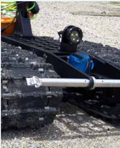
IQNS installed on a Bayonet 250 AUGV.
